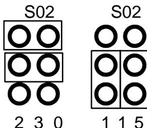
4. To change the AC configuration, remove the jumpers and place them according to the above diagram. Be sure to replace the cover.
